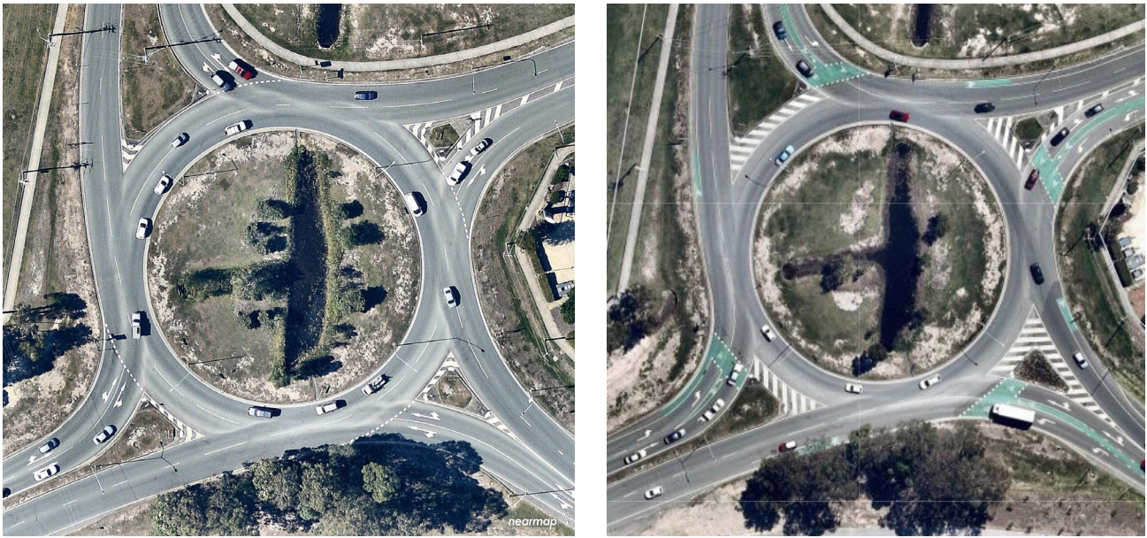
Figure 6 Benabrow Avenue roundabout today [left] and with road diet option design [right] (Source: Moreton Bay Regional Council, ©Nearmap)
